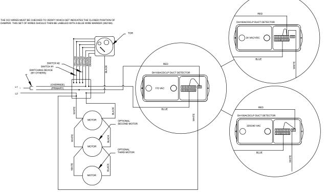
1. CONDUIT RUNS WHICH EXCEED 72\* MUST HAVE GREEN GROUND WIRE. 2. FLEX CONDUIT MUST BE SECURED WITH A CONDUIT CLAMP (48296) WITHIN 12\* OF CONDUIT TERMINATION AT THE HANDI-BOX OR ACTUATOR. CONDUIT RUNS MUST ALSO BE SECURED ALONG SLEEVE AT AMAXIMUM OF 24\* OF CONTERT.
